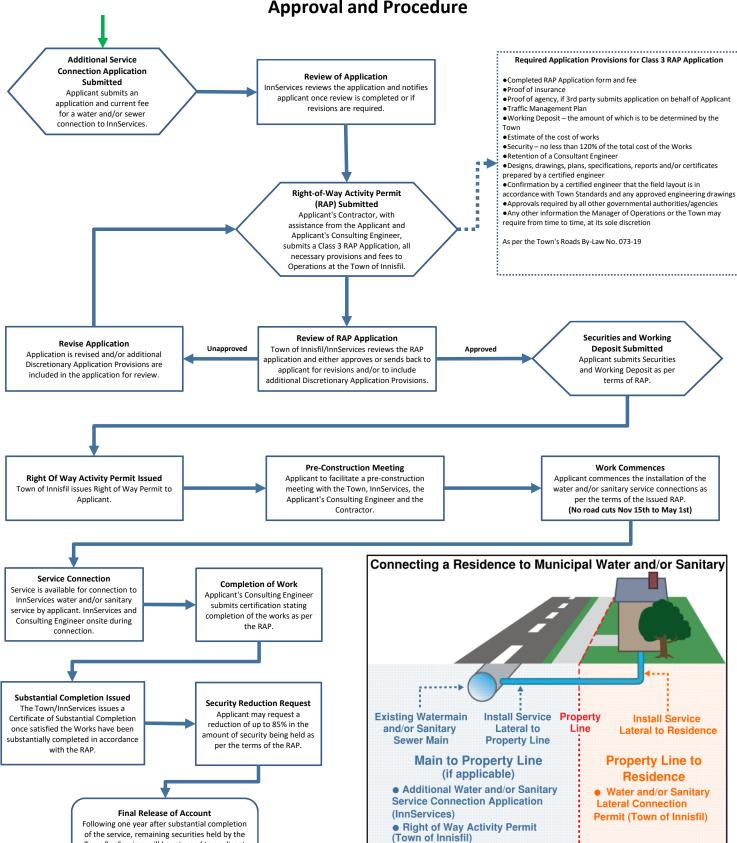
Note - Approval and Procedure for installing service(s) from Main to Property Line as per flow chart. Steps for installing service(s) from Property Line to Residence can be found at the following link: www.innisfil.ca/connecting-to-innservices-water-and-sewer
