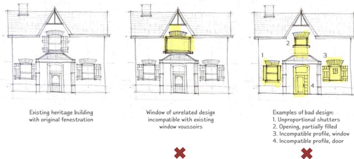
Figure 5-4: Unsympathetic changes in fenestration are not supported
