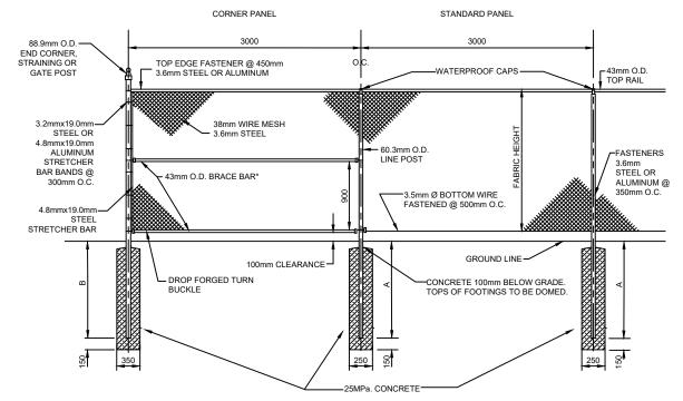
\* ONLY REQUIRED FOR 1800mm FENCE. FIRST AND/OR CORNER PANELS TO HAVE BRACE BAR ALONG BOTTOM INSTEAD OF GUIDE WIRE.
