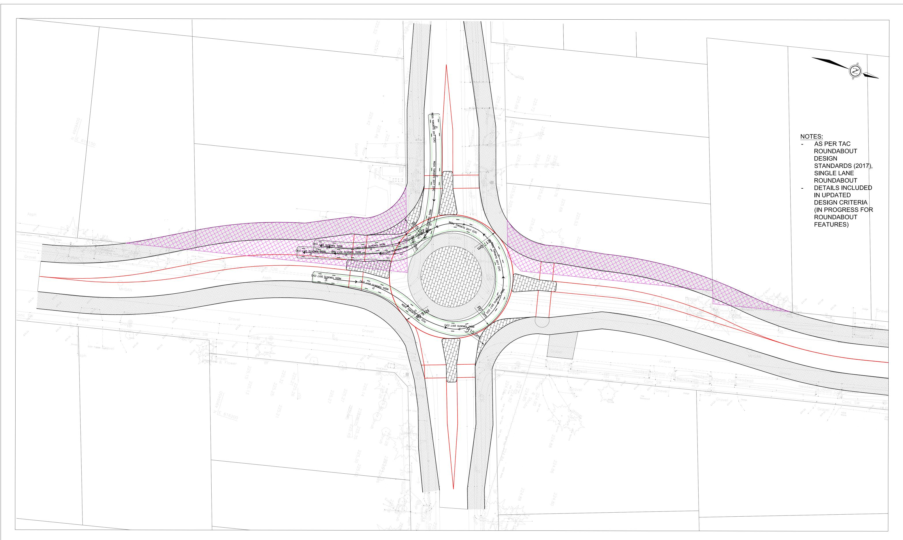
25th SIDEROAD AND 9TH LINE - ROUNDABOUT CONCEPT DESIGN ALTERNATIVE 2a - PASSENGER TURNING ANALYSIS
