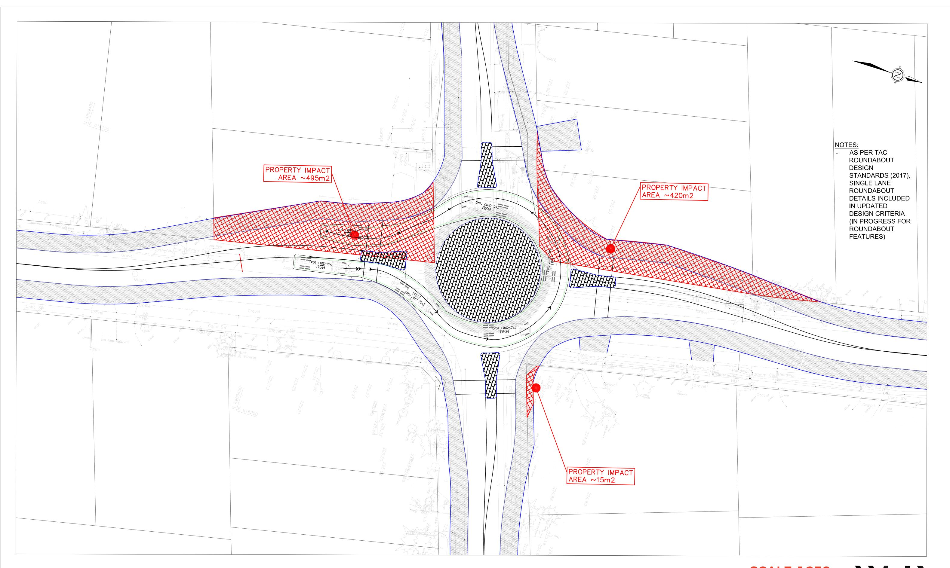
25th SIDEROAD AND 9TH LINE - ROUNDABOUT CONCEPT DESIGN ALTERNATIVE 1 - HSU TURNING ANALYSIS
