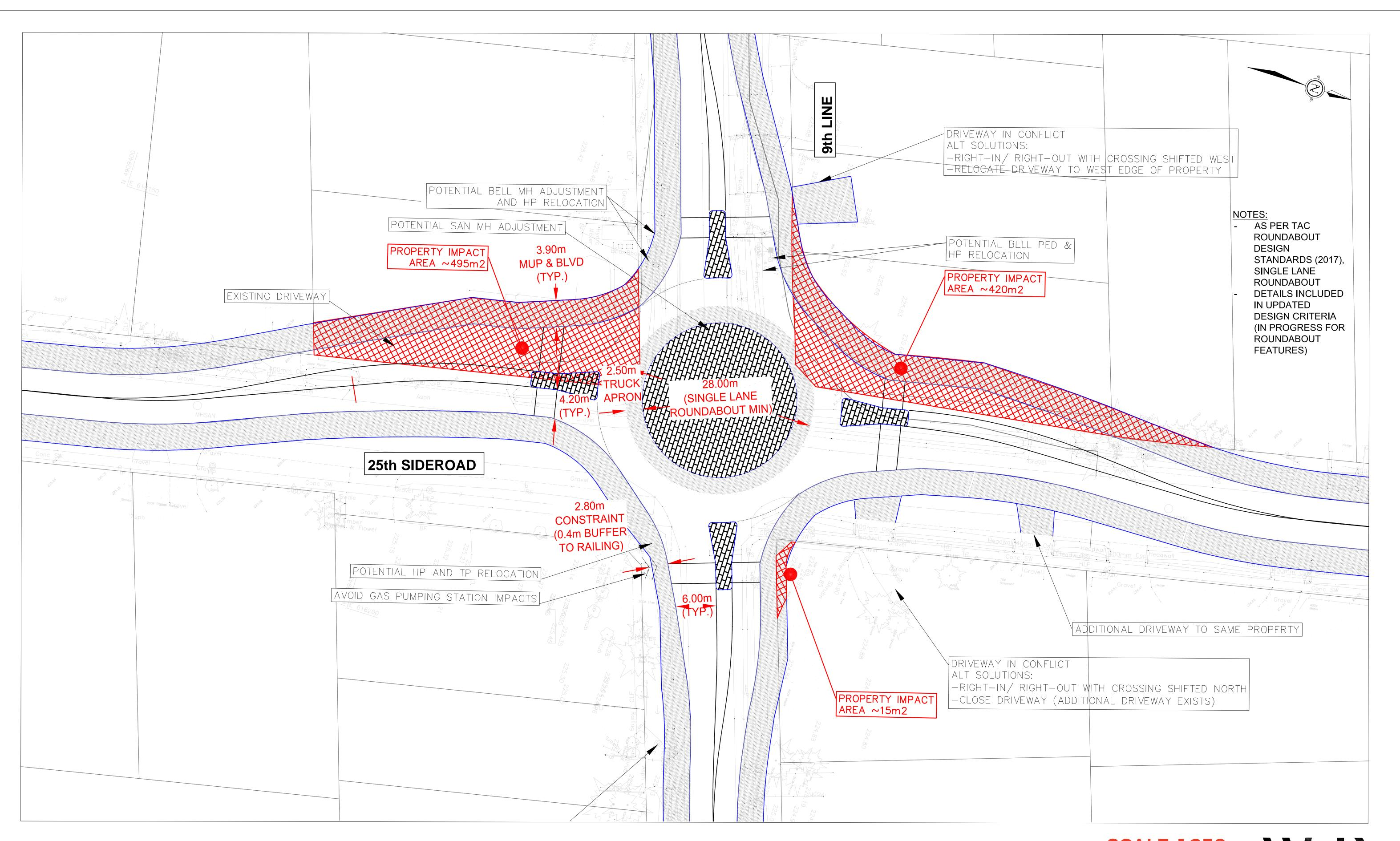
25th SIDEROAD AND 9TH LINE - ROUNDABOUT CONCEPT DESIGN ALTERNATIVE 1 - ICD = 28m
