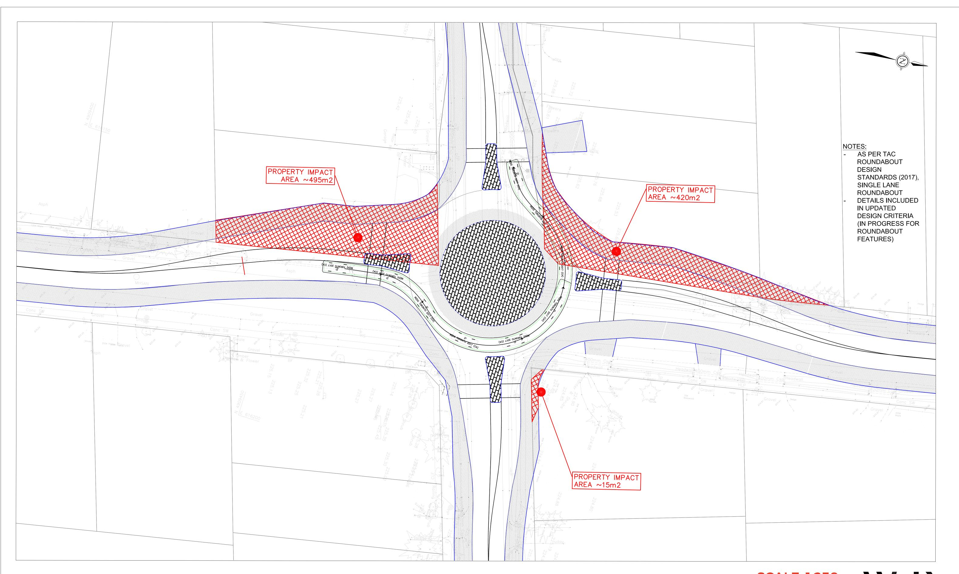
25th SIDEROAD AND 9TH LINE - ROUNDABOUT CONCEPT DESIGN ALTERNATIVE 1 - PASSENGER TURNING ANALYSIS
