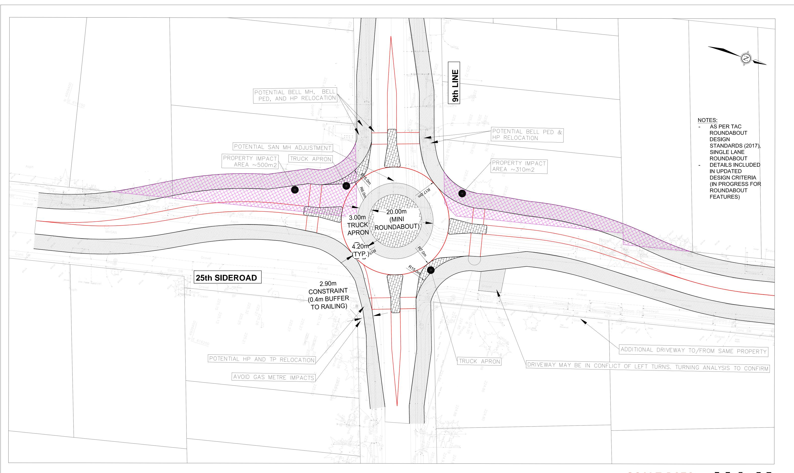
25th SIDEROAD AND 9TH LINE - ROUNDABOUT CONCEPT DESIGN ALTERNATIVE 2a - ICD = 20m
