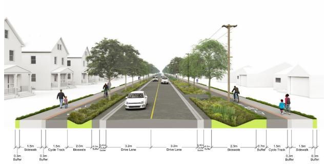
Figure 32: Illustration of a typical cross section for Context 1
