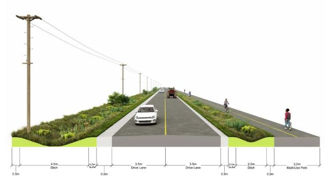
Figure 33: Illustration of a typical cross section for Context 2
