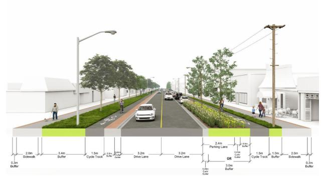
Figure 34: Illustration of a typical cross section for Context 3
