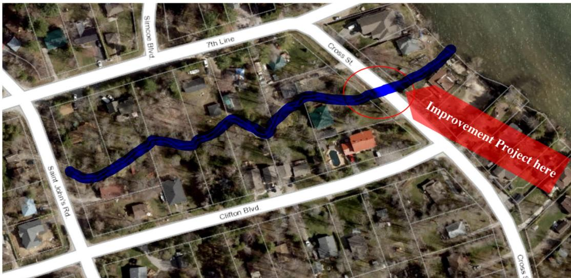
Throughout the design phase, it has been determined that the issues relating to flooding, direction of water and property access would only be slightly improved by moving forward with the preferred alternative of replacing the culvert structure which is in good condition.
