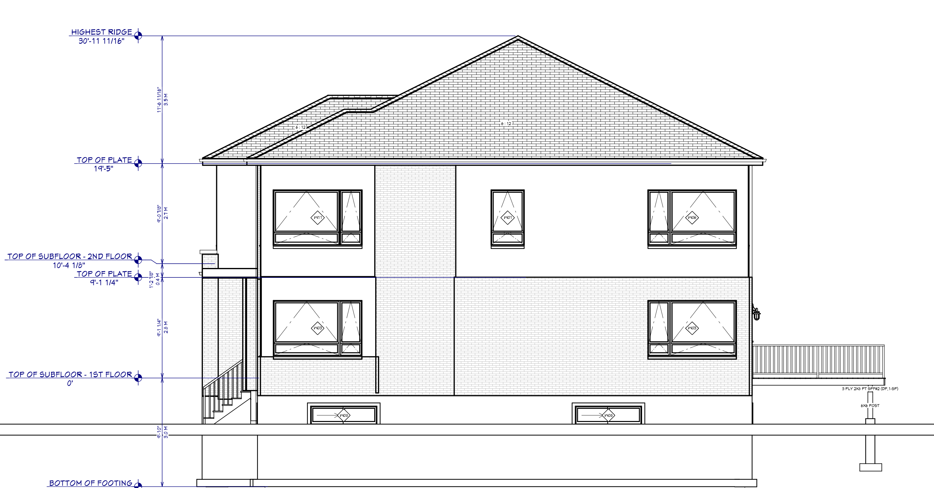
Exterior Elevation Left 3/16 in = 1 ft
