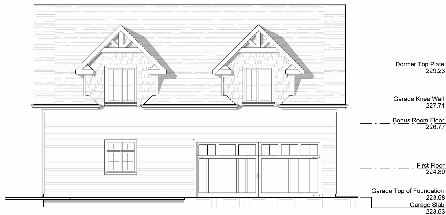
6 Garage South Elevation 1/8" = 1'-0"
