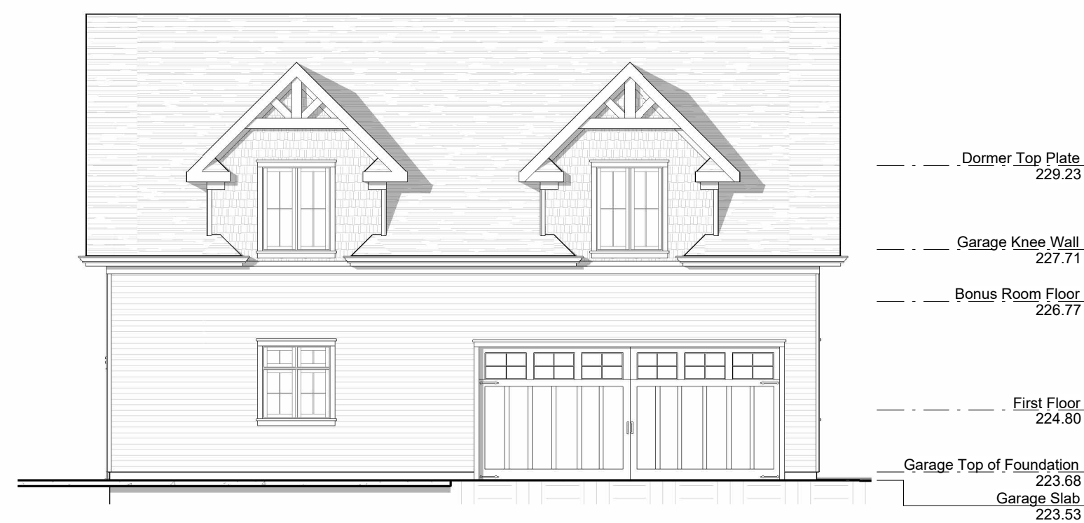
6 Garage South Elevation 1/8" = 1'-0"
