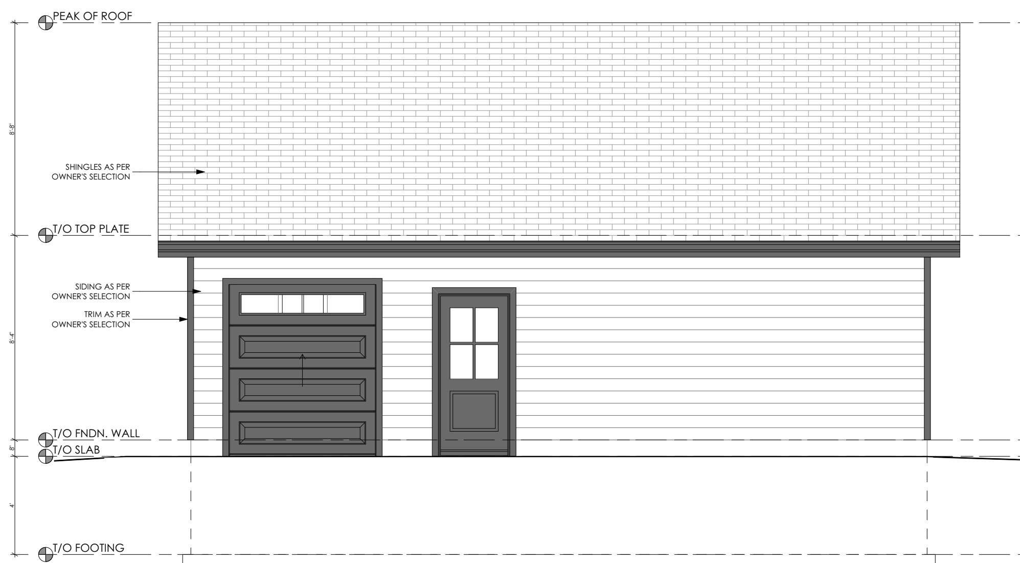
3 NORTH ELEVATION A2.0 SCALE: 1/4" = 1'-0"
