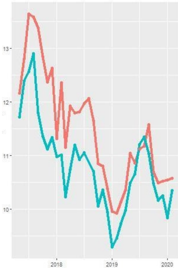
Figure 11. In-Vehicle Travel Times per Trip for Weekdays (blue) and Weekends (red) between May 2017 and February 2020
